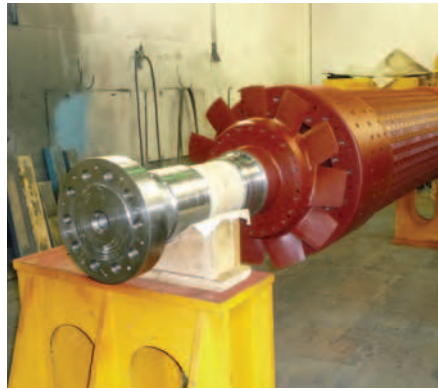
Generator rotor assembly.
