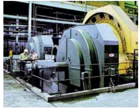
Dual motor load shown for ball mill.
