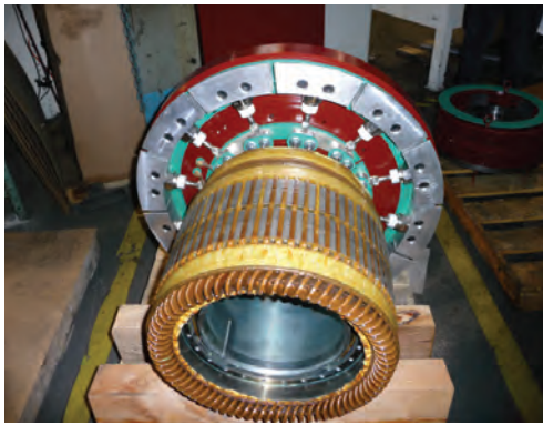
Top row (L to R): PMG with armature and rectifiers; Armature with rectifiers
