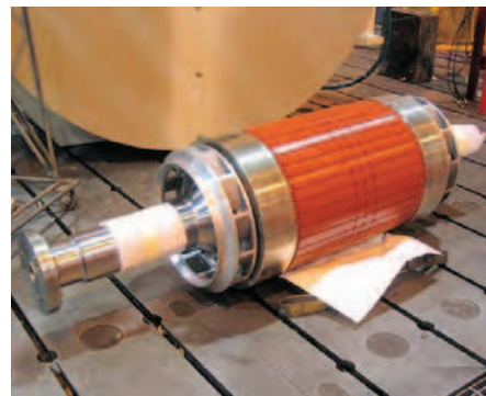
2-pole induction rotor with axial air ventilation.
