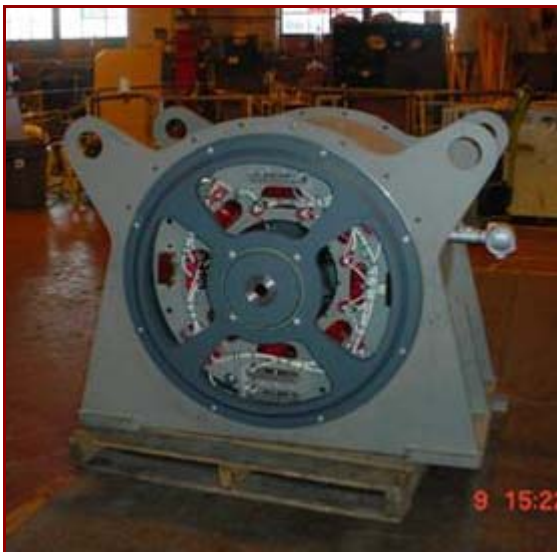
Complete Exciter without Enclosure
