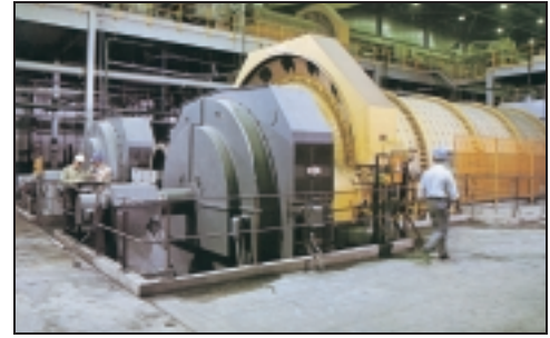
Dual motor load shown for ball mill.
